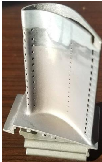
Figure 2.2: Illustration of turbine blade showing holes for cooling [33].
