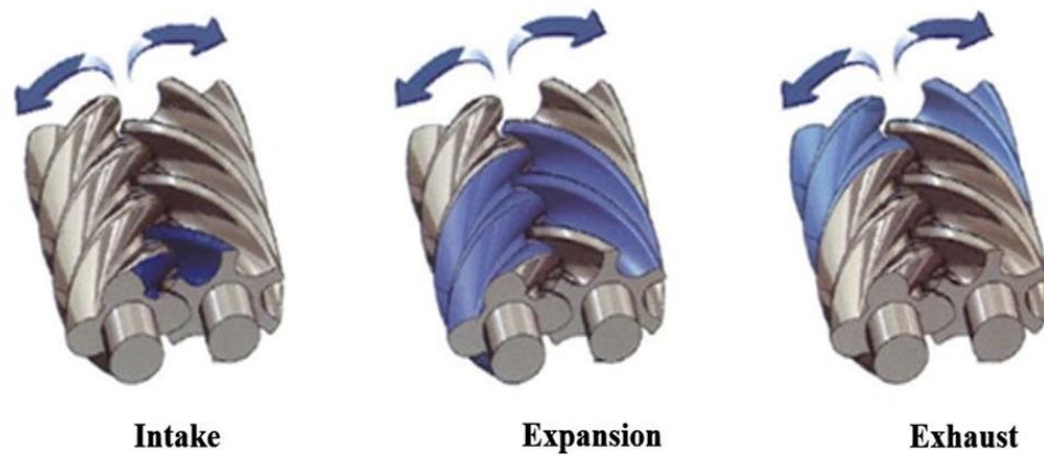
Figure 2.15: Operation of the Screw Expander
