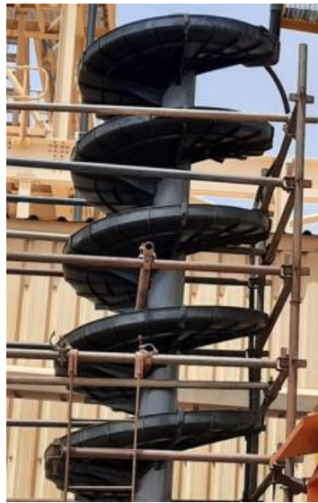
Figure 2.29: A Type H Alicoco spiral installed in the Spiral Rig at GCO
