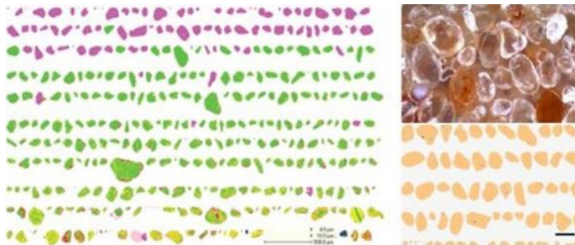
Figure 2.21: Examples of a QEMSCAN image for zircon characterisation (Ramsaywork et al., 2010; Wallmach et al., 2012)
