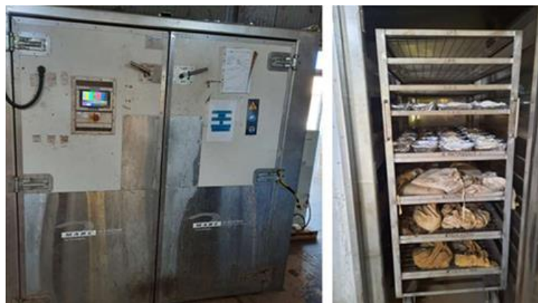
Figure 3.10: A Marc Technologies drying oven (2 m 3 , 415 V, 50 Hz) at GCO laboratory
