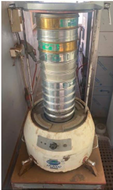
Figure 3.16: A stack of screens on the shaking machine at the GCO Laboratory
