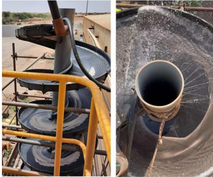
Figure 4.11: Alicoco spiral unable to separate slurry even when water was added at the top of the spiral to reduce beaching
