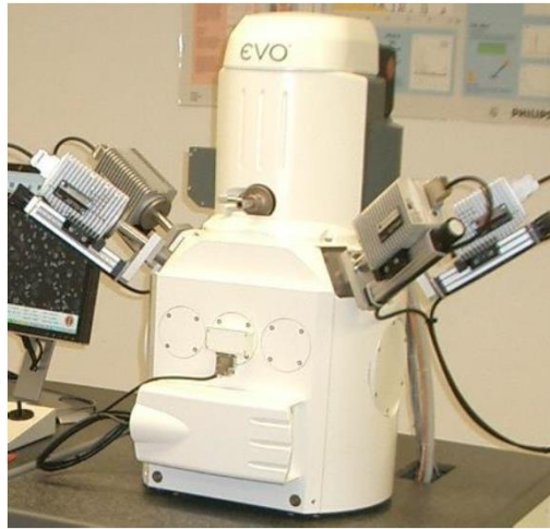
Figure 2.22: A QEMSCAN instrument (Tonzetic et al., 2006)
