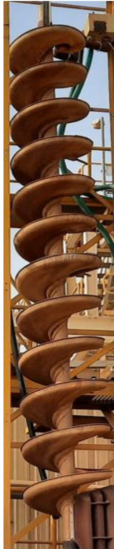
Figure 2.30: The MG12 spiral separator installed at the Spiral Rig at GCO
