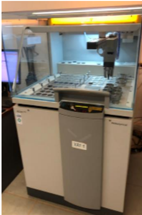
Figure 3.14: One of the two X-Ray Fluorescent (XRF) machines stationed at the GCO Laboratory
