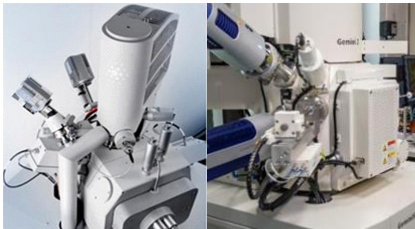
Figure 3.15: A QEMSCAN machine at Eramet Ideas, France
