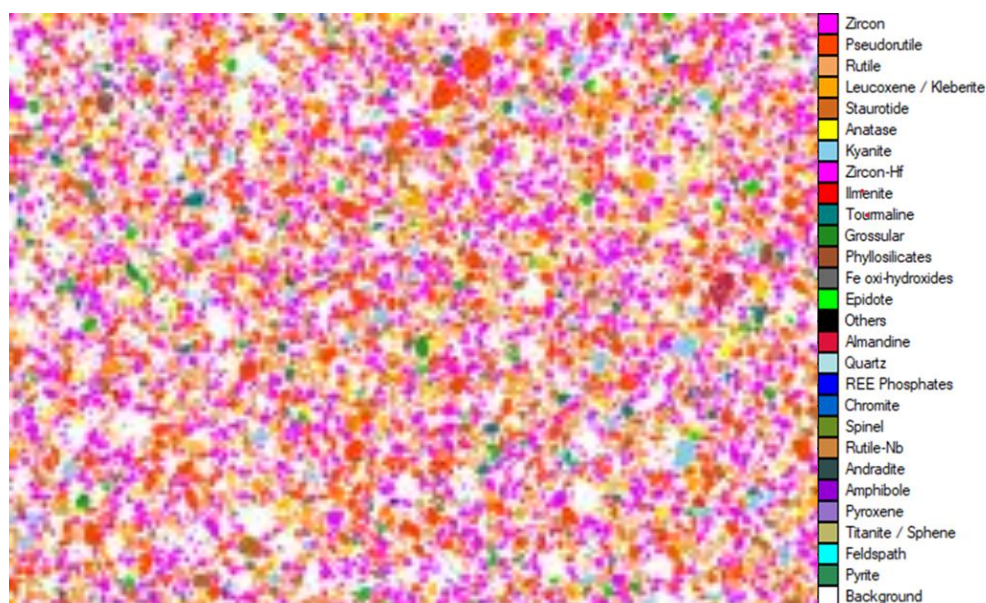
Figure 4.15: The QEMSCAN image of the 35% solids ( 1.36 \text{ g/cm}^3 pulp density) and 78% split concentrate
