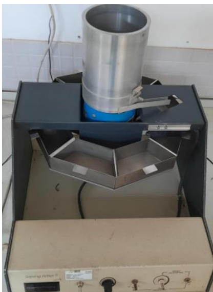
Figure 3.12: A Quantachrome Instruments sieving riffler splitter (220 V, 50/60 Hz) at GCO Laboratory
