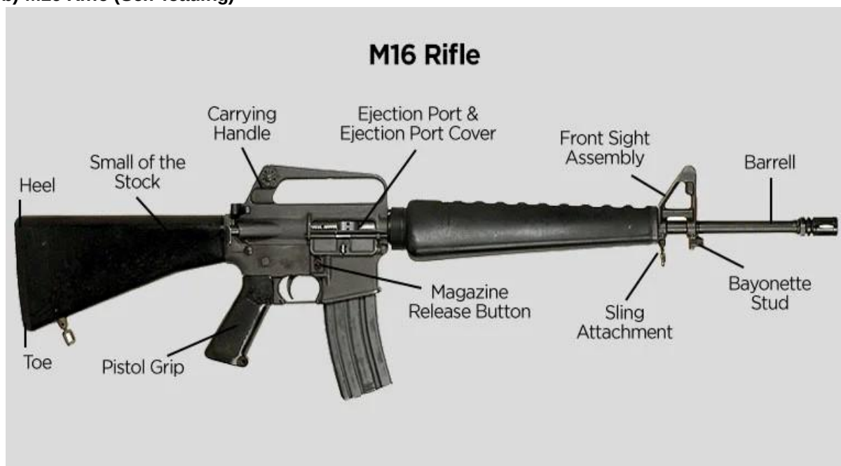
Figure 3. 2: Schematic of a (a) manual-loading and (b) self-loading rifle (Tactical Gear, 2025).
