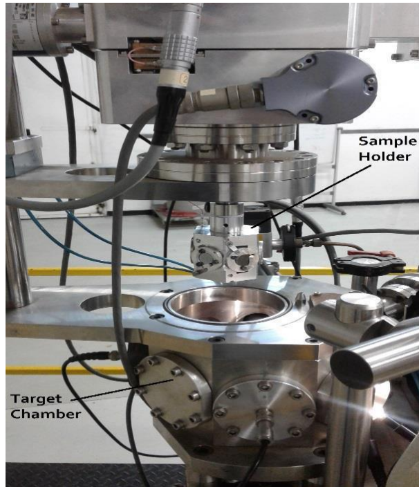
Figure 3.8. Image of the target material sample holder connected to the motorized handler used to move the sample holder on an X- and Y- axis.
