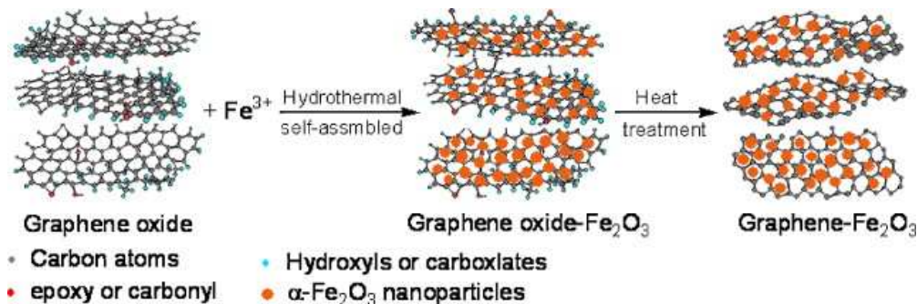
Figure 5.0.2: The structural properties of GO- \text{Fe}_2\text{O}_3 showing homogeneous arrangement of Fe atoms on the edges of GO. Image adapted from Leilei et al. [18].
