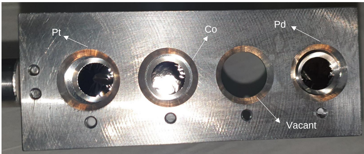
Figure 3.1: Pt, Co, Pd thin foils mounted on a foil holder, with one hole on the holder left vacant.
