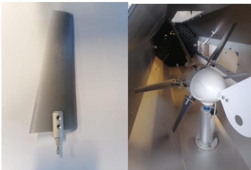
Figure 69: Corrugated Airfoil in a jig to hold it together and fitted in a wind tunnel
