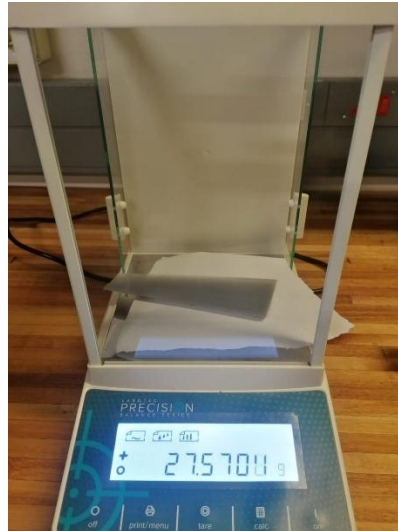
Figure 66: A digital scale used to weigh the 3D printed blades
