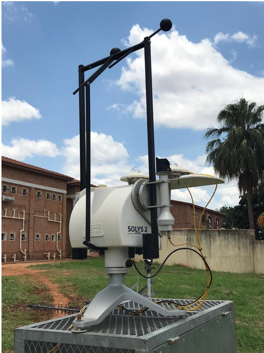
Figure 2.14: A pyrheliometer used to measure the DNI, mounted on the Kipp & Zonen's SOLYS 2 Sun Tracker at Thulamela Information Centre, Thohoyandou, (SAWS station).
