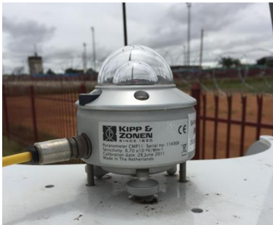
Figure 2.12: Unshaded pyranometer (Kipp and Zonen CMP11 pyranometer) used for measuring GHI at the Polokwane International Airport solar radiation station (SAWS station).
