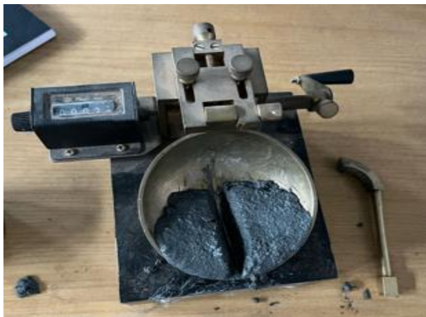
Figure 3.7: An image illustrating a groove made using a Casagrande tool
