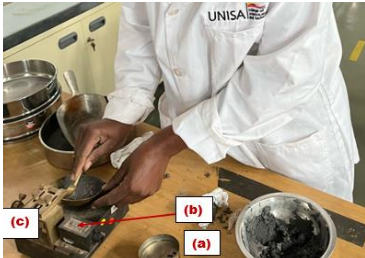
Figure 3.5: Liquid limit apparatus: (a) numbered tin, (b) grooving tool, and (c) Casagrande tool.
