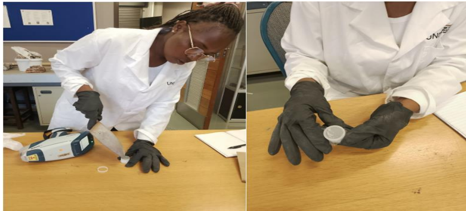
Figure 3.15: Illustrating the placement of tailings into the XRF test container in preparation for the XRF test
