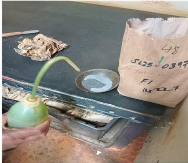
Figure 3.6: A mixing bowl with a tailings specimen and a washer bottle to form a tailing paste
