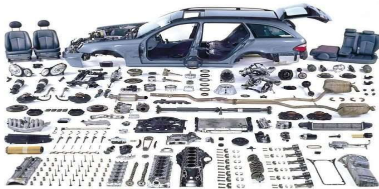
Figure 2.2: Illustrative Example of Exploded View of a Typical Passenger Vehicle.
