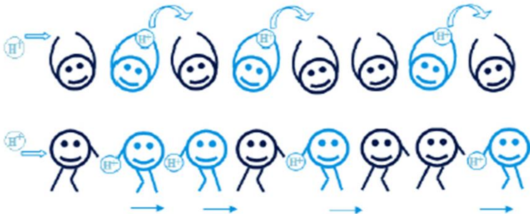
Fig. 2. 4: A schematic representation of the Grotthuss and vehicular mechanisms [30].
