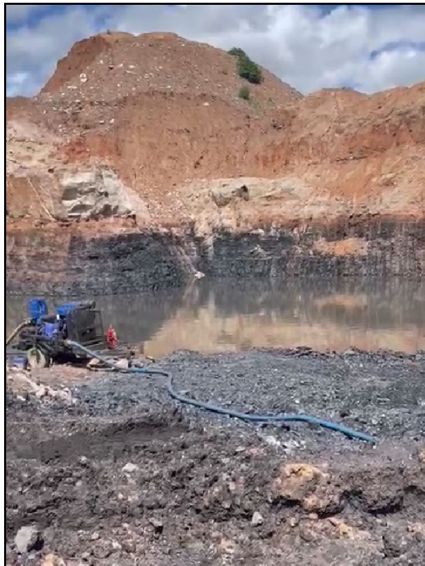
Figure 5.59: Block flooding after Seam 4 extraction in Mine 2
