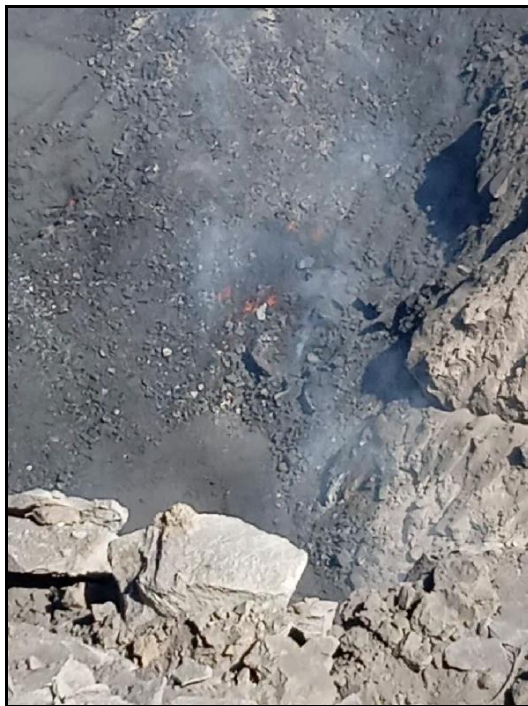
Figure 0.57: Spontaneous combustion of coal pillars at Mine 1
