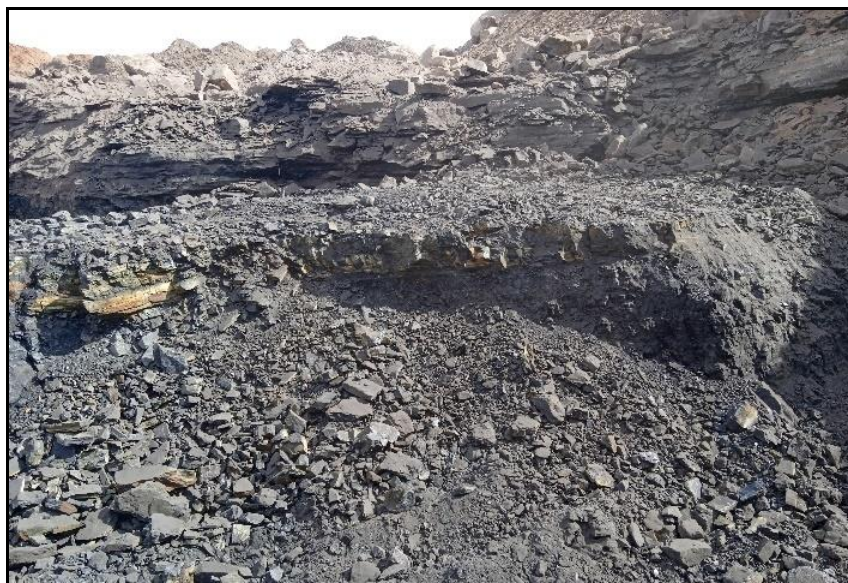
Figure 0.29: Pilot blast of overburden to approximately 0.50 m top of coal
