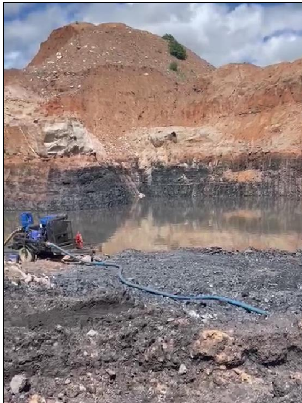
Figure 0.59: Block flooding after Seam 4 extraction in Mine 2
