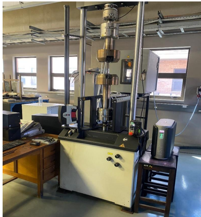
Fig. B8: Tensile testing setup for reinforcing bars
