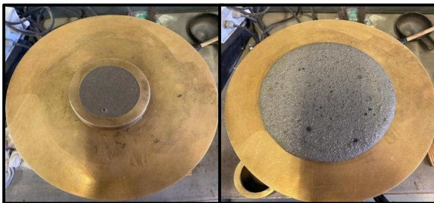
Fig. B2: Flow spread assessment of mortar mixes
