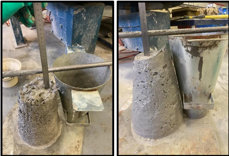
Fig. B5: Measurement of slump for geopolymer concrete mixes
