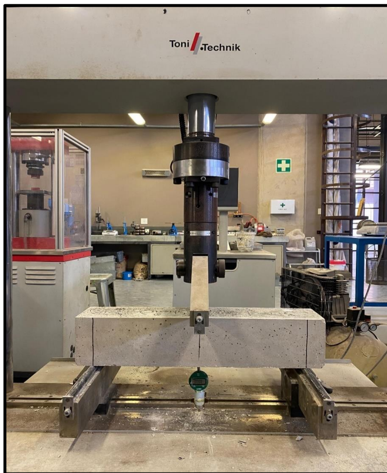
Fig. 3.8: Experimental setup for beam testing
