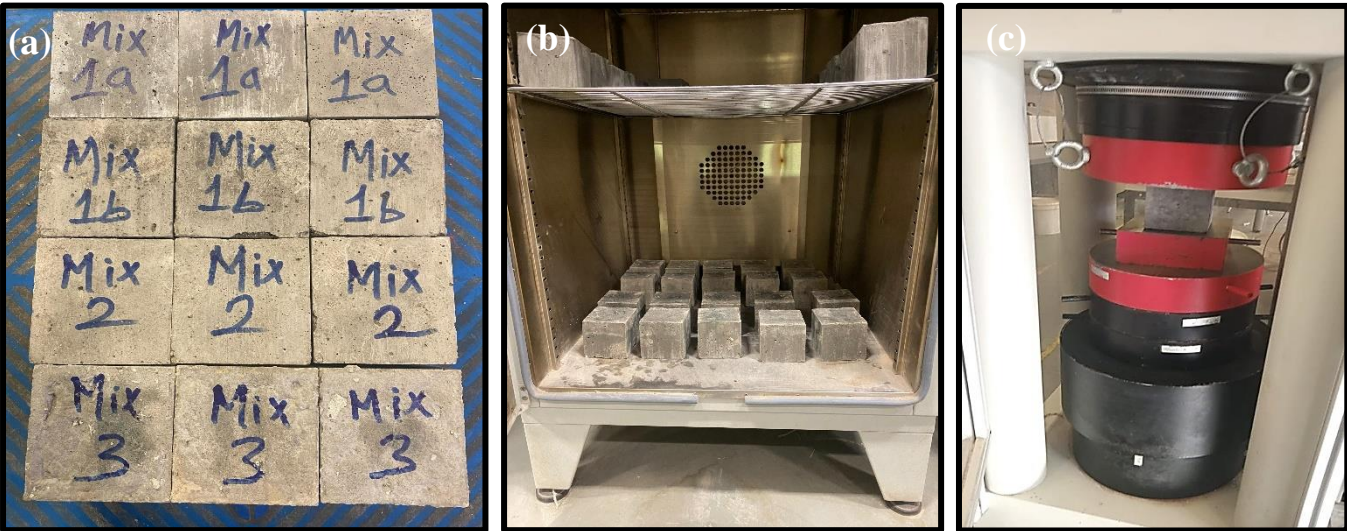
Fig. B6: (a) Hardened concrete cubes after demoulding and (b) oven curing of specimens (c) compressive testing of cubes
