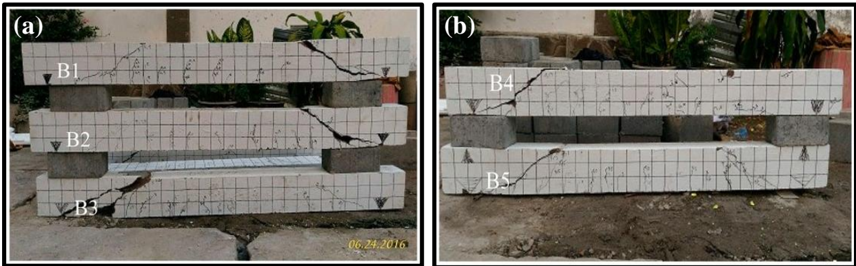
Fig. 2.7: Shear crack propagation in GPC beams cured (a) at room temperature and (b) in seawater (Darmawan et al., 2019)
