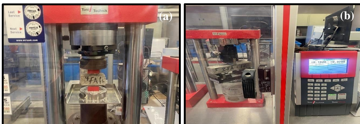
Fig. B3: Strength testing of mortar specimens (a) compressive (b) flexural
