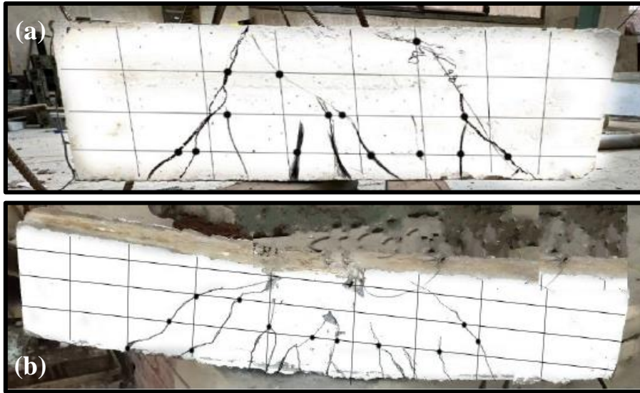
Fig. 2.6: Crack patterns under flexural loading (a) PCC beam (b) GPC beam (Eisa et al., 2022)
