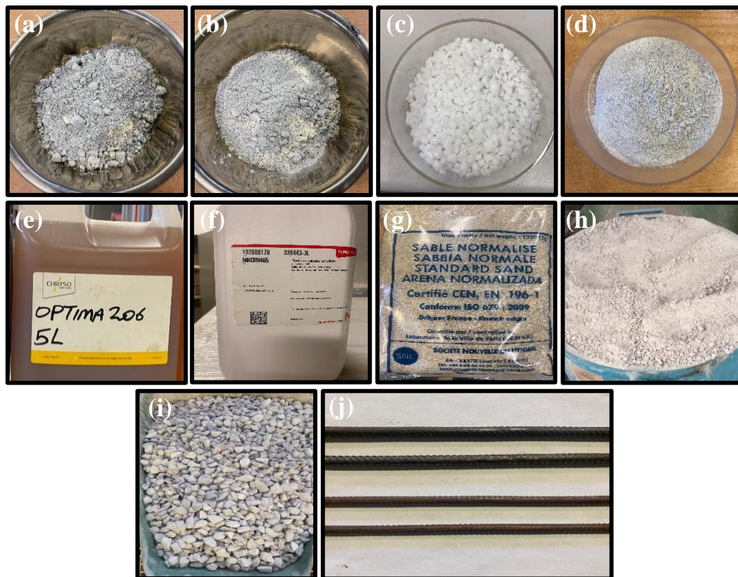
Fig. 3.2: Representative images of (a) fly ash (b) GGBFS (c) NaOH pellets (d) WGP (e) SP (f) CSS (g) Standard sand (h) Crusher sand (i) Coarse aggregates (j) Reinforcing steel bars
