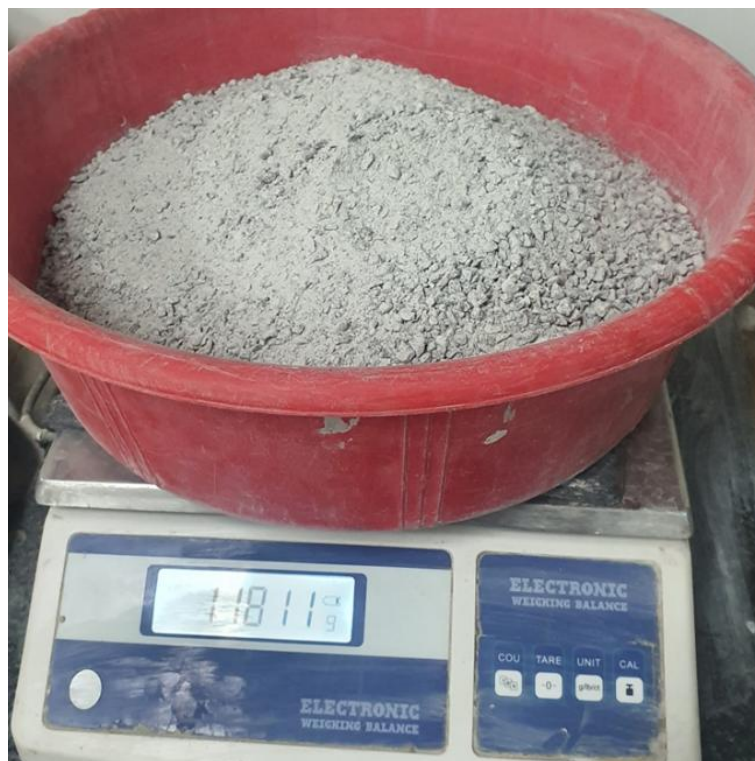
Plate 3.3: Weighing of the crusher sand used in the concrete mixture.
