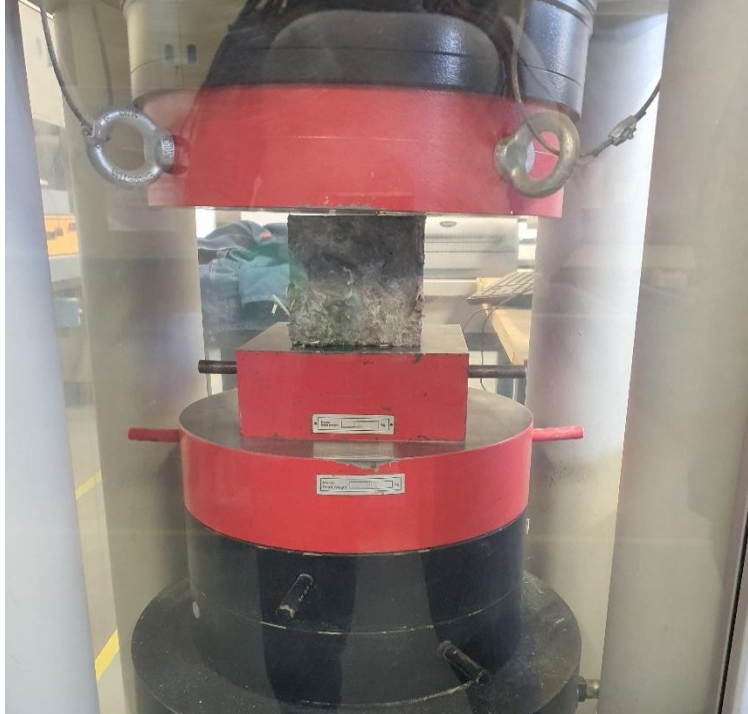
Plate 3.10 :Hydraulic press used for compressive strength testing.
