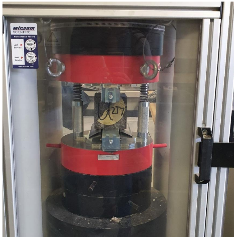
Plate 3.12: Fastened Concrete cube on a Splitting-tensile steel-plates
