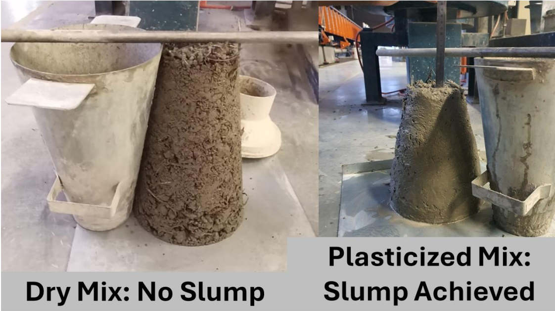
Figure 4.4: Untreated chicken feathers caused no slump, while adding a plasticizer achieved a noticeable slump
