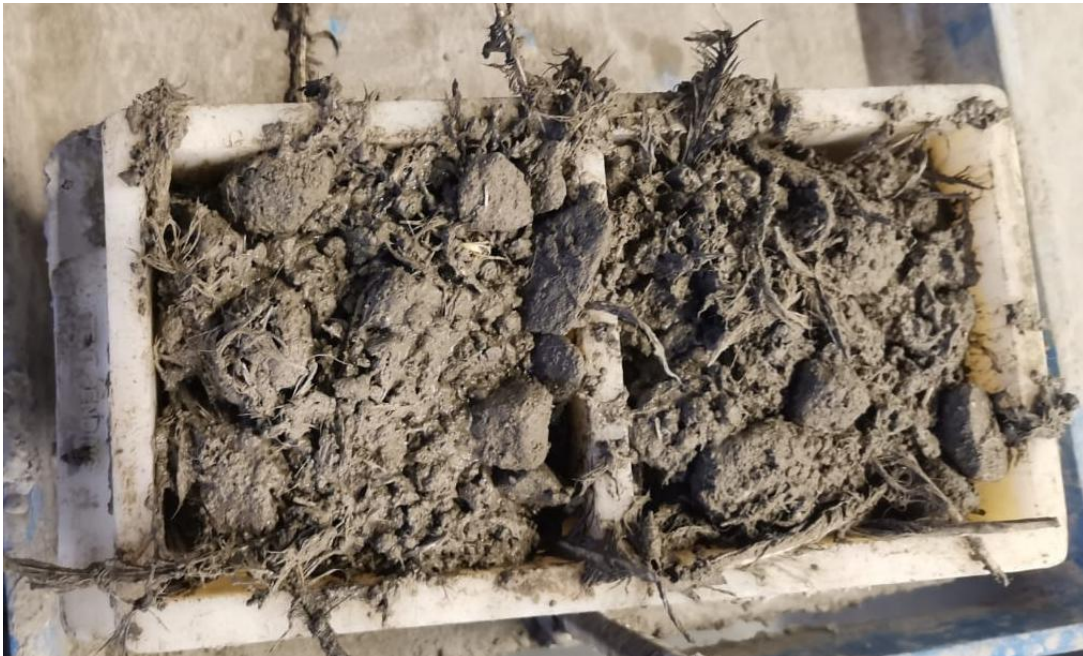
Plate 3.8: Dry concrete mixture in cube mould with incorporated chicken feathers.
