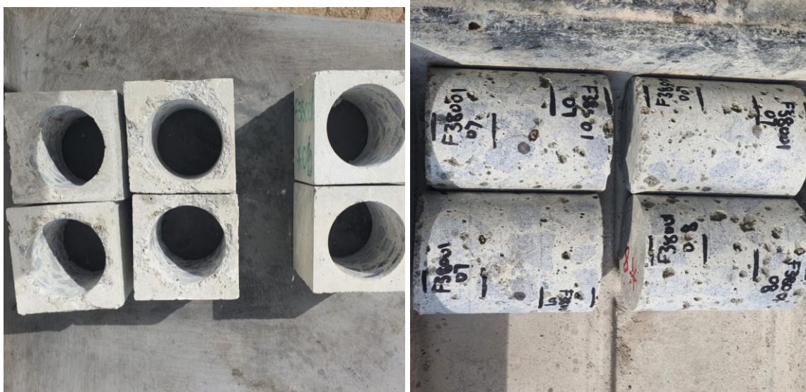
Plate 3 13: Cylindrical concrete cores after coring
