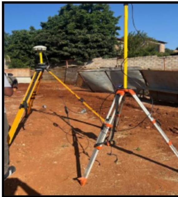
Figure 3.3: Trimble Differential GPS (DGPS) system
