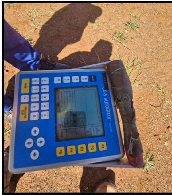
Figure 3.2: Scintrex CG-5 Autograv gravimeter (Scintrex Limited, 2018)
