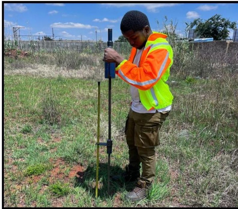
Figure 3.7: Dynamic Cone Penetrometer test
