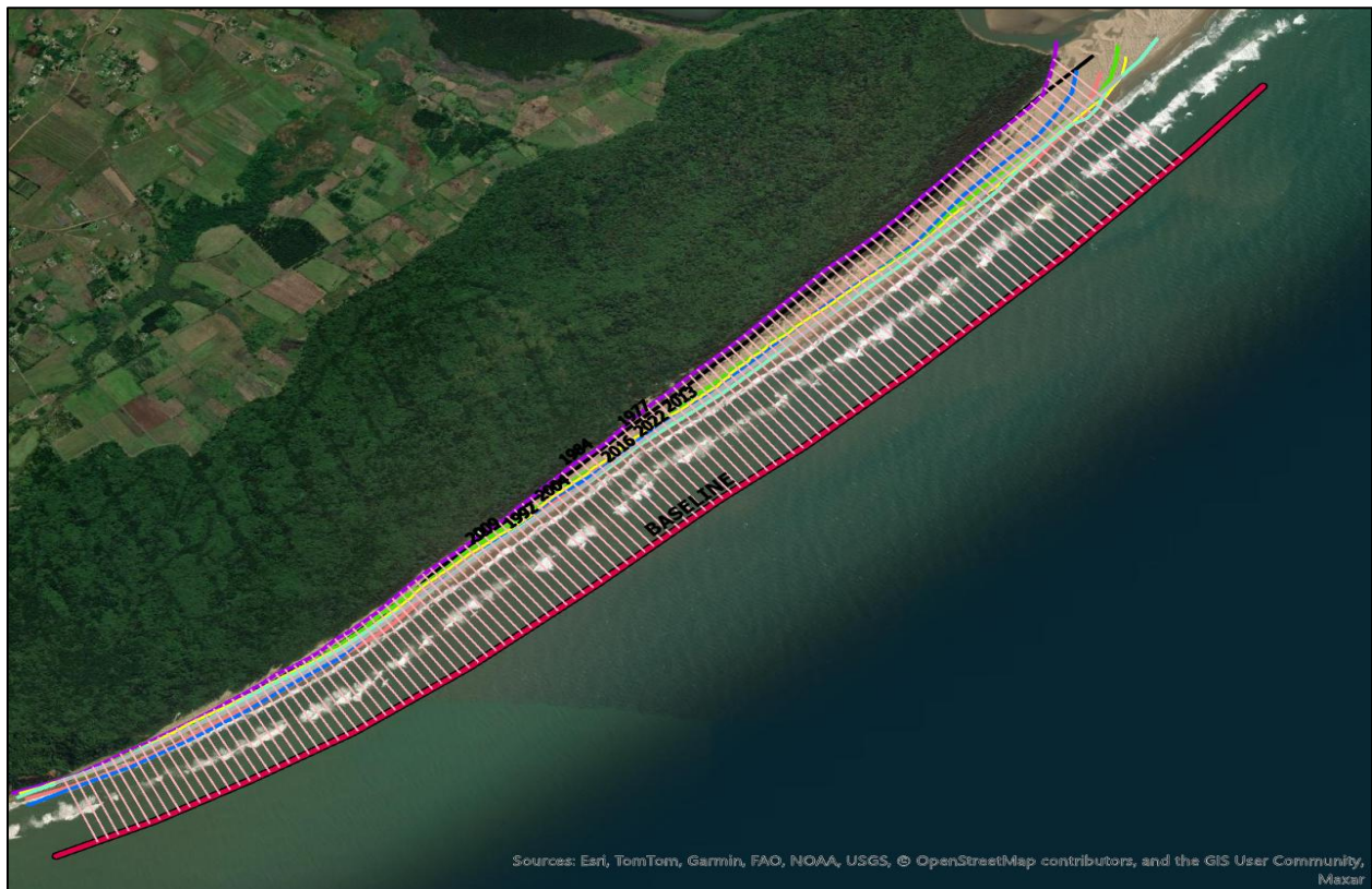
Figure 4.5: The 6.8 km stretch of beach known as uMhlathuze Estuary showing 123 transects spaced 50 m apart, the reference baseline (red), with digitized historical shoreline positions (multicolour).
