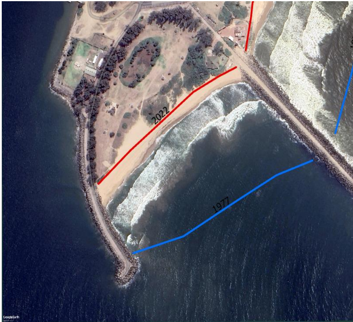
Figure 5.3: The Net Shoreline Movement for Alkantstrand between 1977 and 2022 was 167.8 m in a landward direction (erosion) according to the DSAS calculations.
