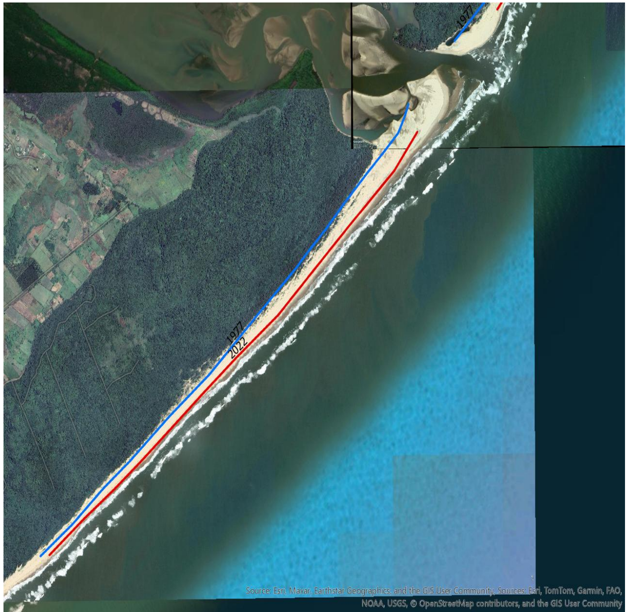
Figure 5.2: The Net Shoreline Movement for uMhlathuze Estuary between 1977 and 2022 was 93.06 m in a seaward direction (accretion) according to the DSAS calculations.
