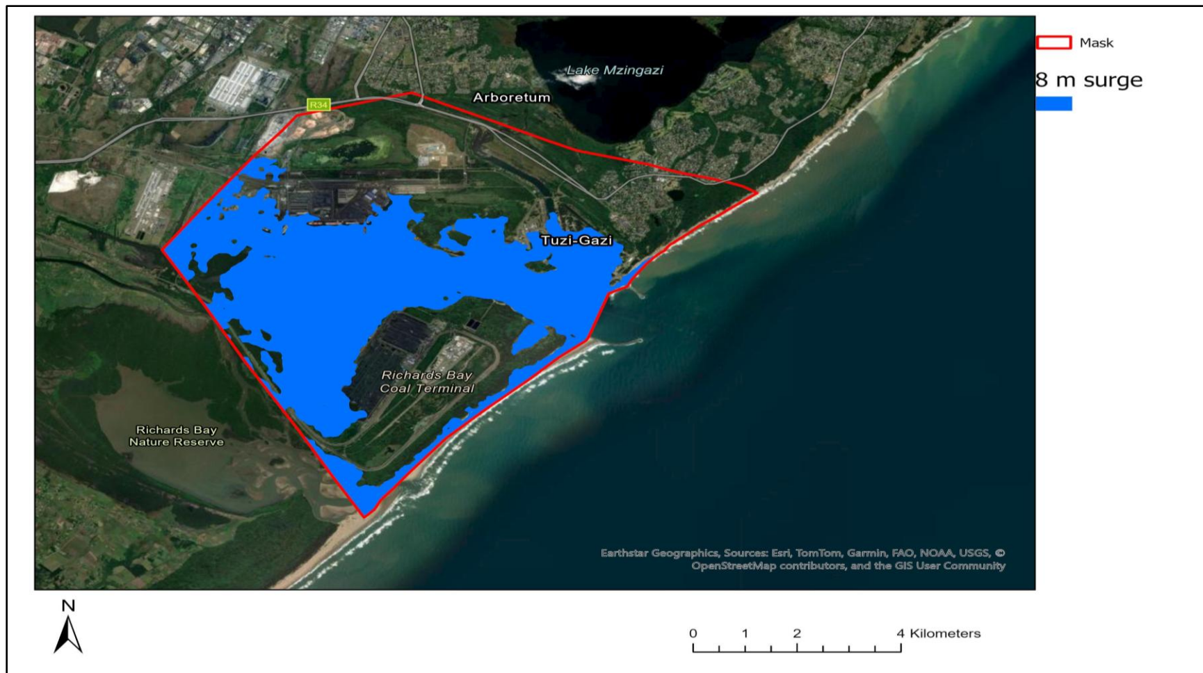
Figure 4.16: Inundation Model depicting the floodable areas of the study site when experiencing a storm surge level of 8 m.
