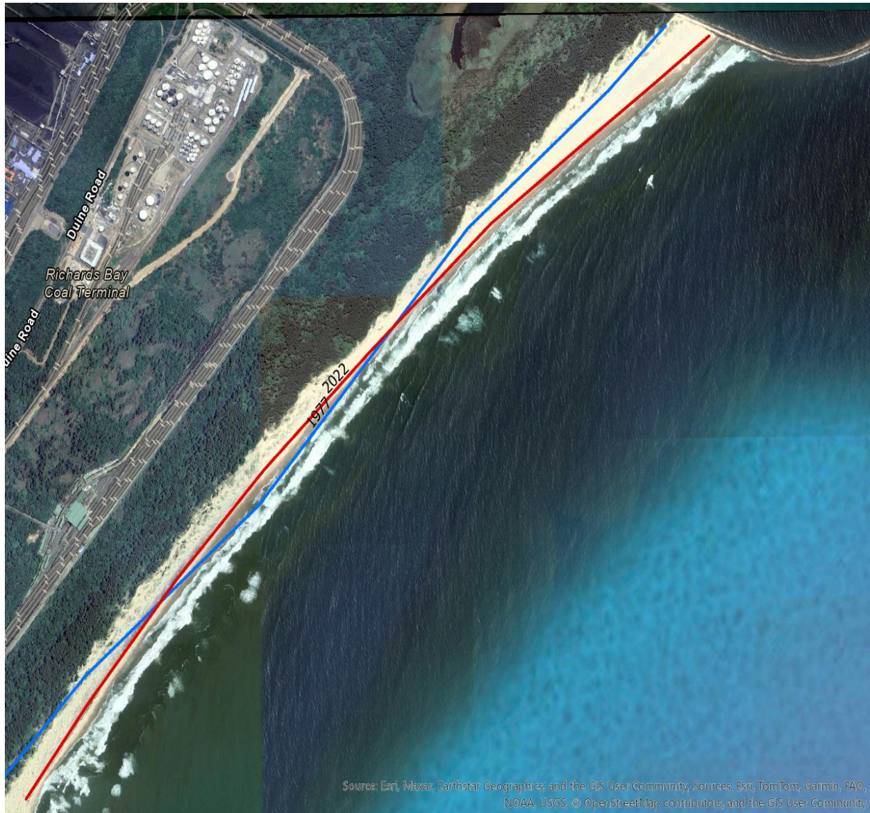
Figure 5.1: The Net Shoreline Movement for South Dunes between 1977 and 2022 was 98.90 m in a seaward direction (accretion) according to the DSAS calculations.
