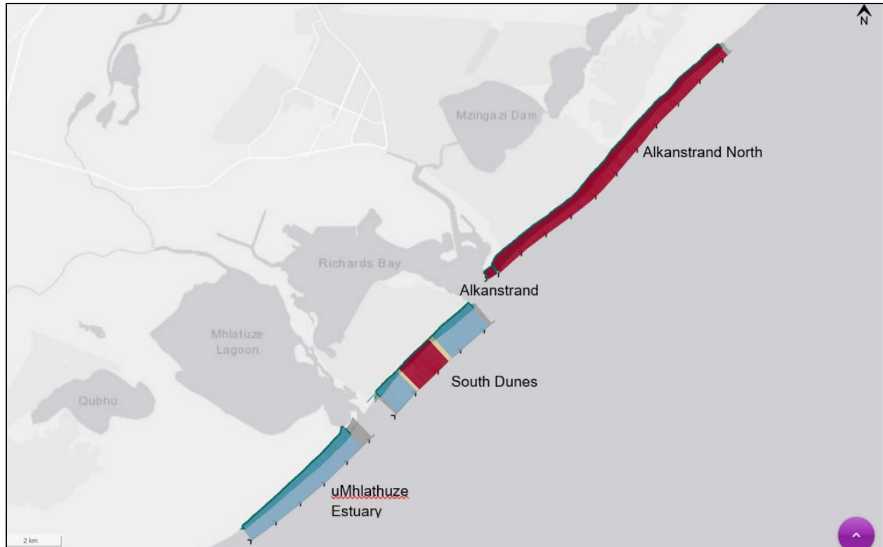
Figure 4.3: Summary of the results map from DSAS showing erosion in red , accretion in blue and no change in yellow .
