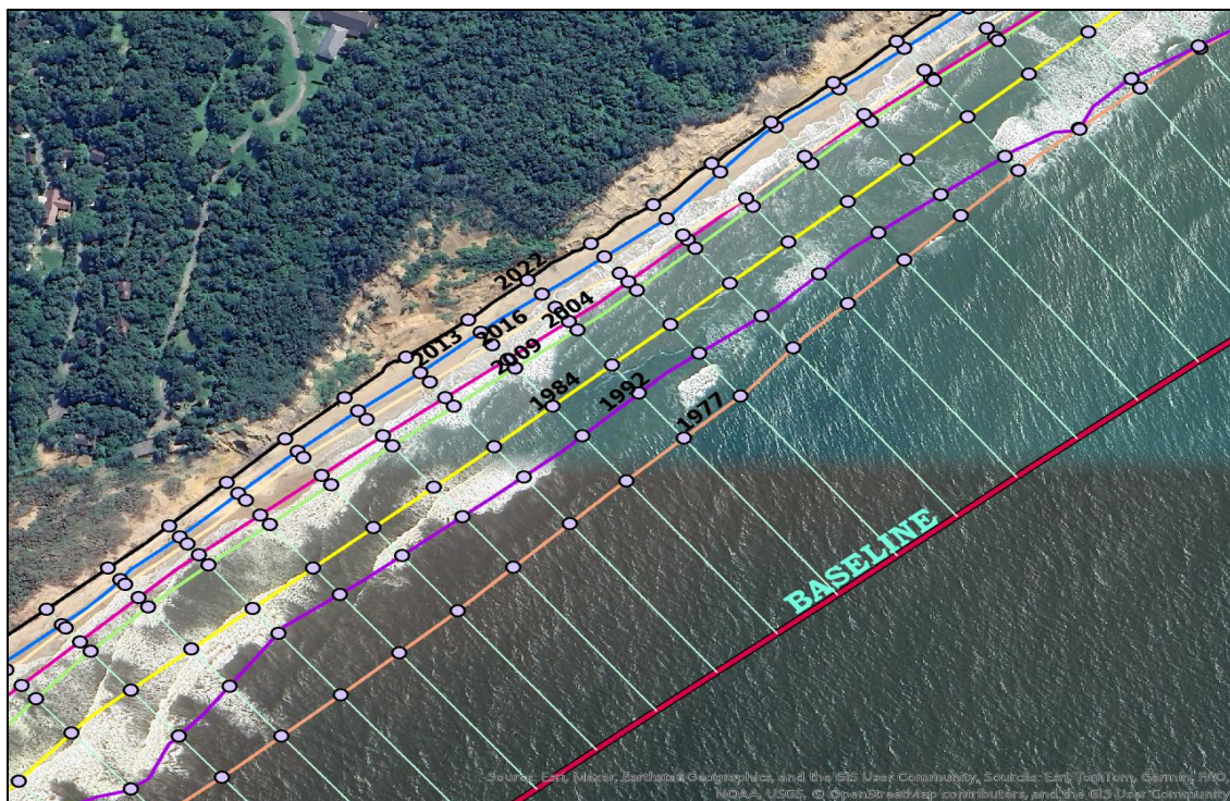
Figure 4.4: A section of digitized shorelines of Alkanstrand North showing DSAS-generated transects (spaced 50 m apart) with reference baseline (red) and historical shoreline positions (multiple colours). The measurement distance from the baseline to each intersect point is used in conjunction with the corresponding shoreline date to compute rate of change statistics.
